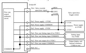
If the high accuracy of the control is necessary, setting flow rate voltage is COMMON (Pin.8), and the flow rate output is COMMON (Pin.7) on the power side. Please do not connect the power COMMON (Pin4).
