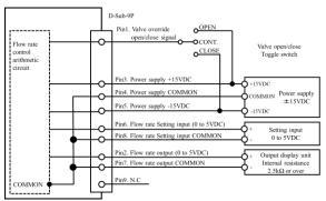
Do not connect. Flow rate setting signal COMMON[8], Flow rate output signal[7], and Power supply COMMON[4] in the power supply unit.
