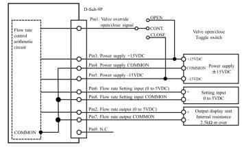
Do not connect. Flow rate setting signal COMMON[8], Flow rate output signal COMMON[7], and Power supply COMMON[4] in the power supply unit.
